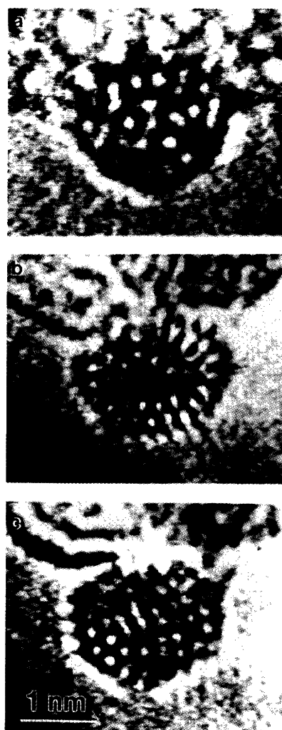
Fig. 1. Single-frame video tape HRTEM images of a small gold cluster rotating on an amorphous carbon support. The cluster is ca. 2 nm in diameter with around 400 atoms. The icosahedral structure is imaged with near five-fold symmetry in (a) and with three-fold symmetry in (b). The typical two-fold symmetry can be seen in (c).
